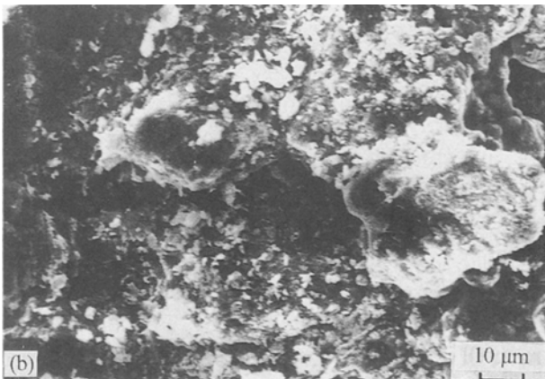
Figure 5 Comparison of scanning electron micrographs of sol-gel-derived (a) HT and (b) LT as-dried powders.
